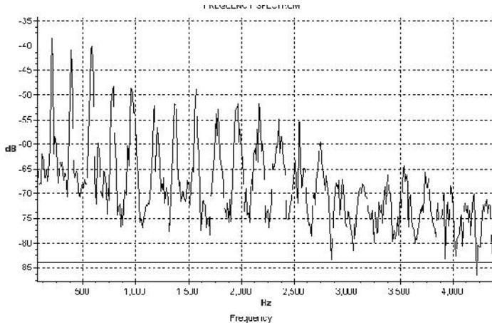
The Arachapu is a very powerful stroke and elicits a very large number of harmonic overtones. Note that the near harmonic overtones are all strong and comparable in strength. Further, the second harmonic is almost equal in strength to the third harmonic. The placement of the edge of the hand along the diameter during the strike forms a nodal diameter and thus the second harmonic is excited more
