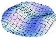
3. **The second overtone mode:** In this mode, the drum head vibrates such that there are two nodal lines due to variation in the angular direction. This mode is designated as the (2,1) mode. The frequency of this mode is  $2.135f$ .
