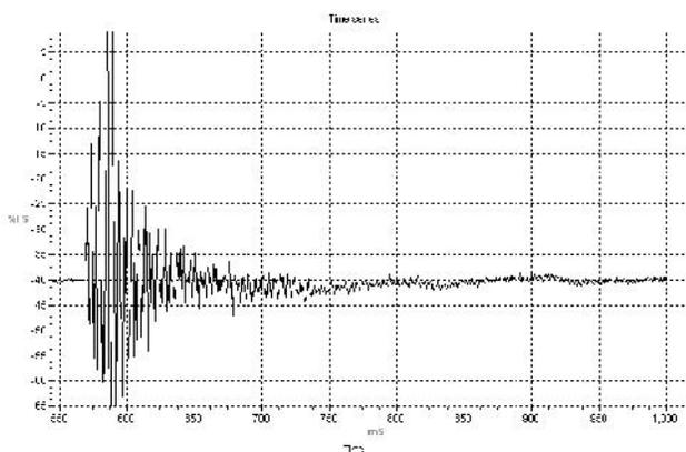
The adjoining figure represents the waveform of the Mrudanga Chapu. (Note that this is an oscilloscope pattern and not a spectrum plot.) It can be clearly seen that after the *Attack phase*, the amplitude of vibration varies in a cyclical fashion while generally decreasing in an exponential pattern. This amplitude modulated sound gives us the perception of the distinct “chapu” sound of the Mrudanga. Some people have called this the “snare” sound. This is
