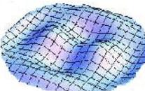
6. **The fifth overtone mode:** This mode is designated as (2,2). The drum head vibrates in such a way that there are two nodal lines and one nodal circle. The frequency of this mode  $3.5f$ .
