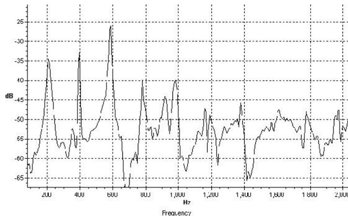
The striking feature of this spectrum is the strong third harmonic. The fundamental is suppressed quite substantially (it is about 8 times smaller than the third harmonic). The second harmonic is also fairly strong and even the higher harmonics are stronger as compared to the Dheem case. The strong presence of the second and third harmonic enables us to hear the missing fundamental at
