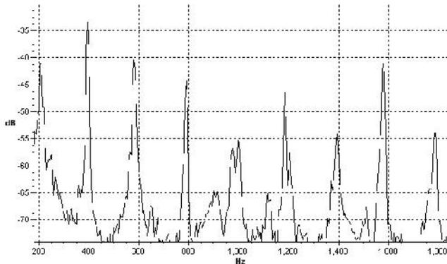
The Chapu is yet another powerful stroke that elicits a very large number of harmonic overtones. Note that all the near harmonic overtones are strong and comparable in strength. The second harmonic is very strong and the fundamental is about 16 times smaller than this. The actual fundamental is at 209.6 Hz, which is about 1.06 times the perceived tonic frequency. The other frequencies in the spectrum are
