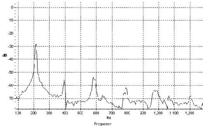
This spectrum clearly shows a prominent fundamental at 214.7 Hz. The second harmonic is at 395 Hz. In the case of sounds like Meetu, the perceived fundamental is taken to be half of this at 197.5 Hz. (Notice that this is close to the standard, G pitch equal to 196 Hz.) Thus the actual fundamental is about  $214.7/197.5=1.07$  times the perceived fundamental. The other frequencies in the spectrum are the second harmonic at 395
