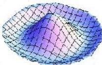
4. **The third overtone mode:** This mode is designated as (0,2). There is no variation in the angular direction but there is a nodal circle formed due to variation in the radial direction. The frequency of this mode is  $2.29f$ .
