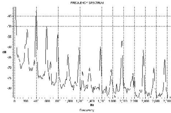
It can be clearly seen that the out of tune fundamental has decreased 10 times at this point in time. This difference will get further accentuated with the passage of time until all components decrease to un-audible levels. A similar behavior is observed in the case of other pitched sounds as well. Thus we perceive the correct fundamental in each case except in case of Dheem where the fundamental is very much stronger than the other components.
