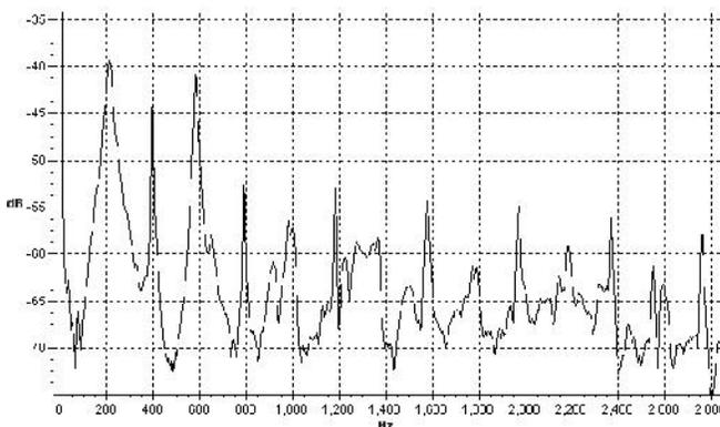
During the Dhim stroke, the Karane is hit at its edge using the index finger. In the Mrudanga, most of the vibrational energy is confined to the Karane area and striking this will produce a number of overtones. The fundamental, second, and third harmonic are all strongly excited and this gives a rich tonal texture to this stroke. The fundamental is at 211.7 Hz, which is about 1.08 times the tonic frequency. The other
