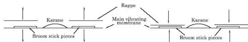
Phase when the two membranes are moving apart. This produces strong un-hindered vibrations.
