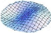
2. **The first overtone mode:** In this mode, the drum head vibrates such that there is one nodal line due to variations in the angular direction. This mode is designated as the (1,1) mode. The frequency of this mode is  $1.593f$ .
